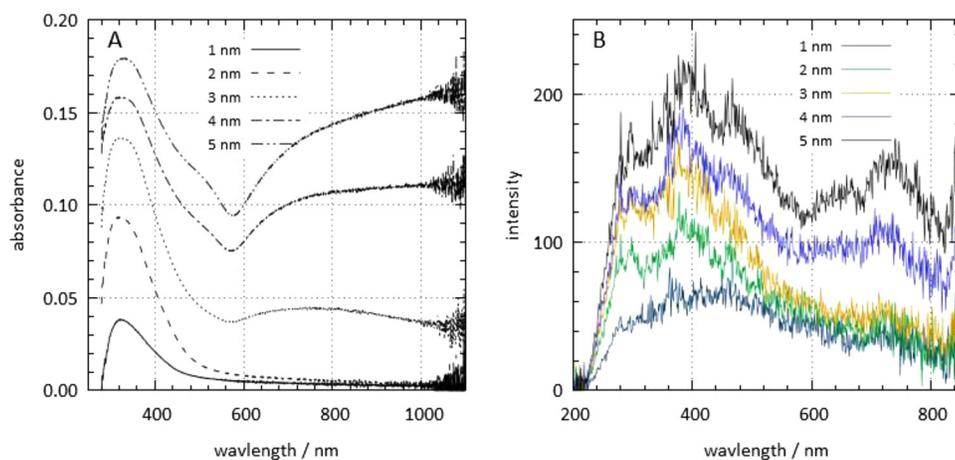
FIG. 1. (a) Absorbance spectra recorded on microscopy slides coated with different thicknesses of Cu. (b) Synchronous scattering spectra,  $\lambda_{ex} = \lambda_{em}$ , recorded on the Cu slides.
