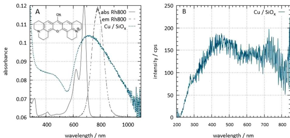
FIG. 2. (a) By coating the 4 nm thick Cu films with a 4 nm layer of SiO<sub>x</sub>, it is possible to prevent oxidation of Cu. This protective coating has a large effect on the plasmon band. The absorbance and emission spectra observed for Rh800 dissolved in methanol are also shown. The chemical structure for Rh800 is shown in the inset. (b) Synchronous spectra recorded for the SiO<sub>x</sub> coated slides. Note that the films are dry.
