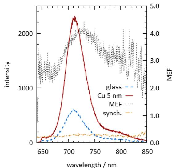
FIG. 3. Spectra recorded for Rh800 dissolved in glycerol and sandwiched between glass slides (control) and between glass copper slides (sample). The calculated MEF response is shown together with the synchronous spectra.
